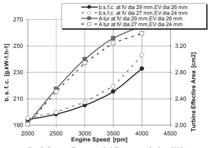
Fig. 7. Engine efficiency with different size of valves [12]
