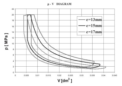
Fig. 9. A simulated pressure diagram of a high pressure steam engine of rotational type
