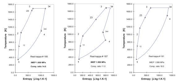
*Fig. 8. Engine cycles using heat regeneration between 34-344 and 12-2. Cycles have the same efficiency despite changes in compression ratio*
