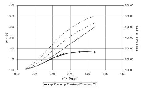
Fig. 6. Dependence of power-balanced compressor and turbine pressure ratio for certain turbine lay-out at given temperature of exhaust gas upstream a turbine. Flow-rate dependence on pressures upstream turbine and downstream compressor explains the demand on low-loss exhaust aftertreatment facilities
