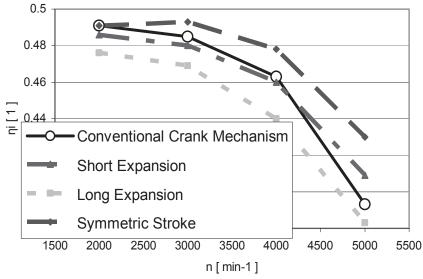
Fig. 5. Cycle efficiency for trapezoidal pattern of piston motion with interruptions at TDC and BDC
