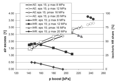
Fig. 4. Air excess and share of isochoric heat supply for different limits of maximum pressure and variable boost pressure
