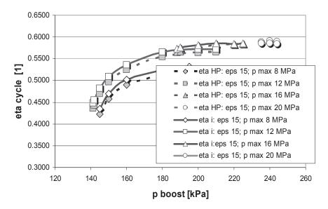
*Fig. 3. Cycle efficiency without cooling losses for high pressure part (HP) and the whole cycle (eta i) including turbocharger losses*
