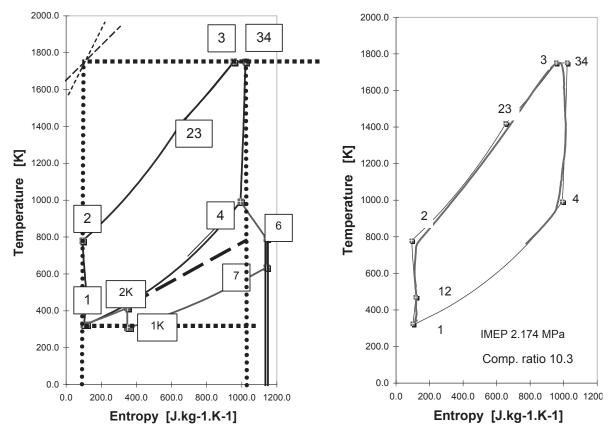
Fig. 1. T-s diagram of a turbocharged ICE
